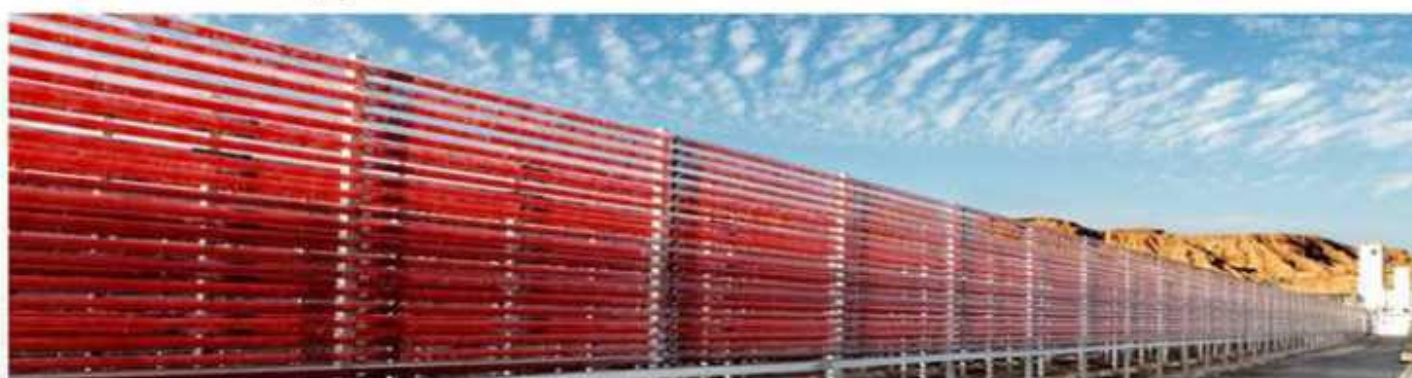
Fig. 2. Outdoor photobioreactor for the cultivation of Haematococcus pluvialis for the production of astaxanthin (source: https://www.scientistlive.com/content/high-quality-microalgae-products ) functions and properties of biopigments
